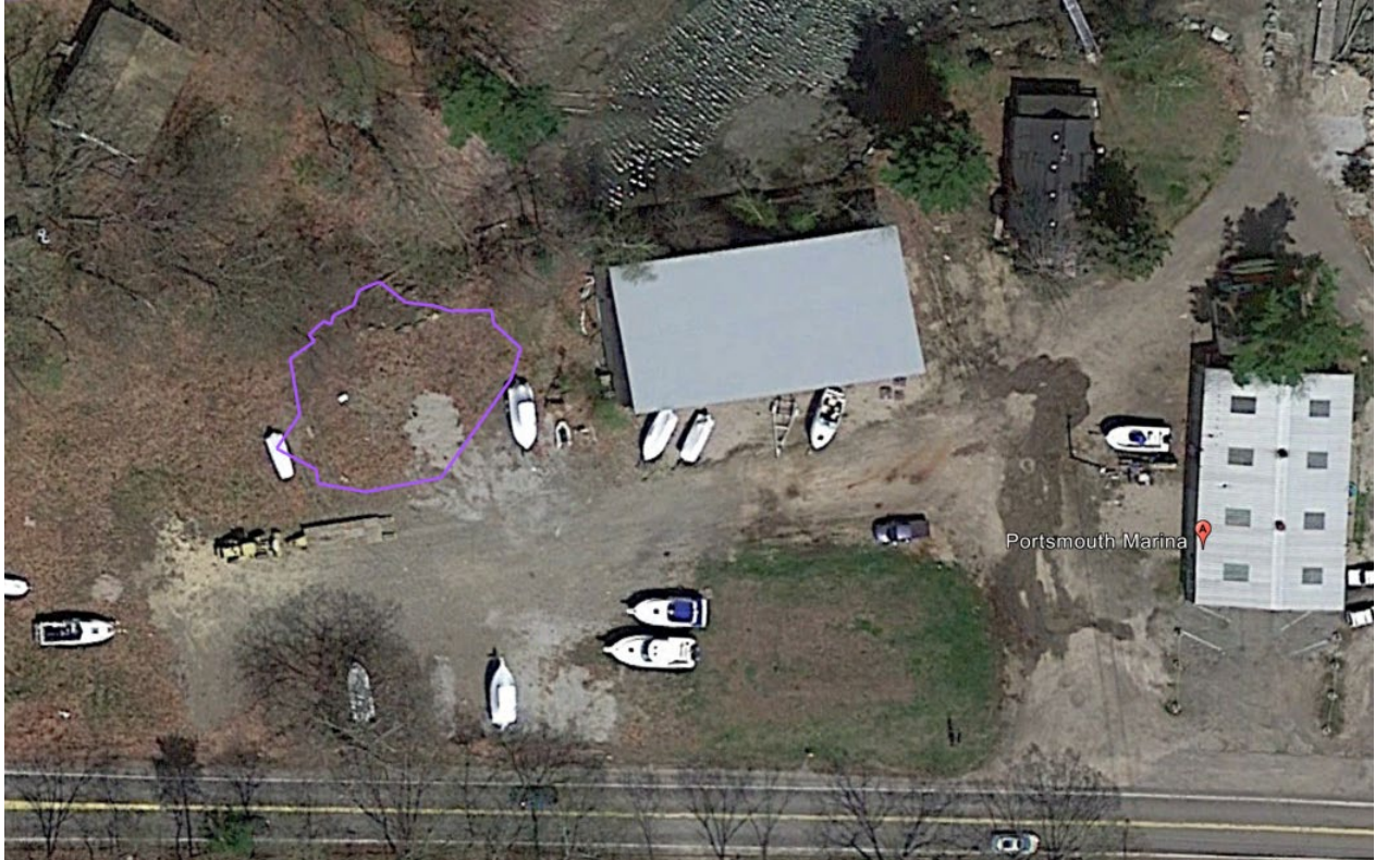
Photo 4: May 2015 Google Earth Image – Approximate 2016-2017 PCB excavation extents outlined in purple. Evidence of 2014 excavation is seen at bottom right of excavation extents.
